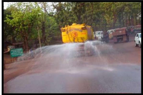
**Photos showing mobile water tankers engaged for dust suppression**
