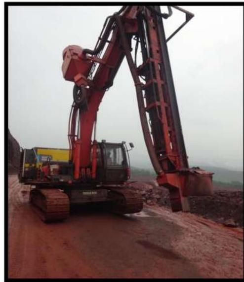
**Photo Showing Excavated Mounted Drilling Machine equipped with dust extractor &
