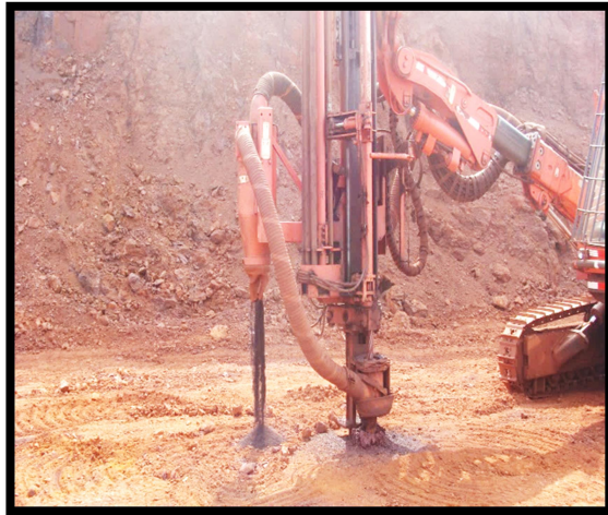
Photo Showing DP 1100 Hydraulic Drilling Machine equipped with dust extractor & wet drilling mechanism
