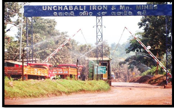
Photos showing automatic fixed sprinkler installed at mines permanent Haul road
