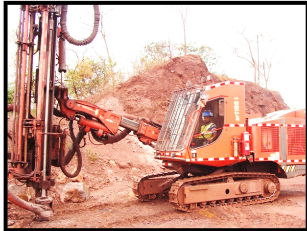
Photo Showing DP 1100 Hydraulic Drilling Machine equipped with dust extractor & wet drilling mechanism
