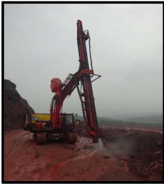
Photo Showing Excavated Mounted Drilling Machine equipped with dust extractor & wet drilling mechanism
