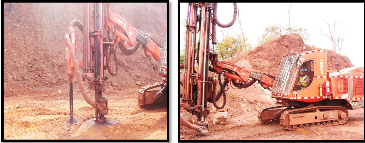
Photo Showing DP 1100 Hydraulic Drilling Machine equipped with dust extractor & wet drilling mechanism
