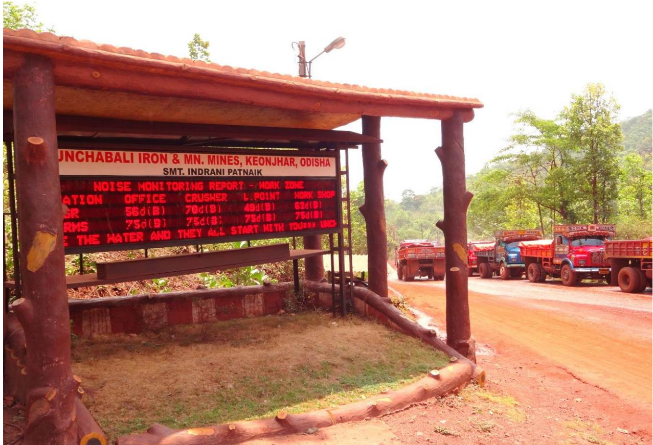
Photo Showing Electronic Display board placed in the mines entrance gate to display the Environmental parameters
